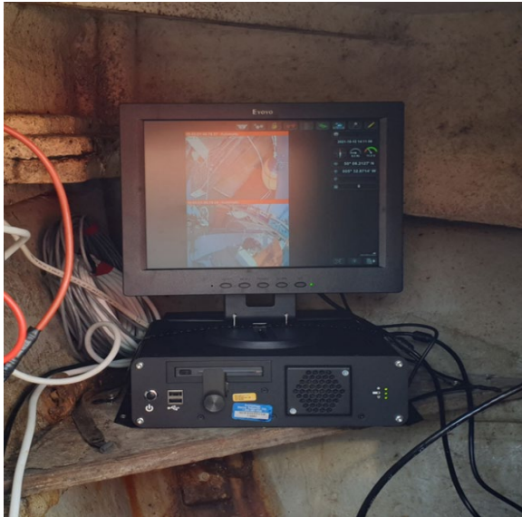
Figure A3 – The AMR V5 electronic monitoring system implemented on a small inshore UK vessel
