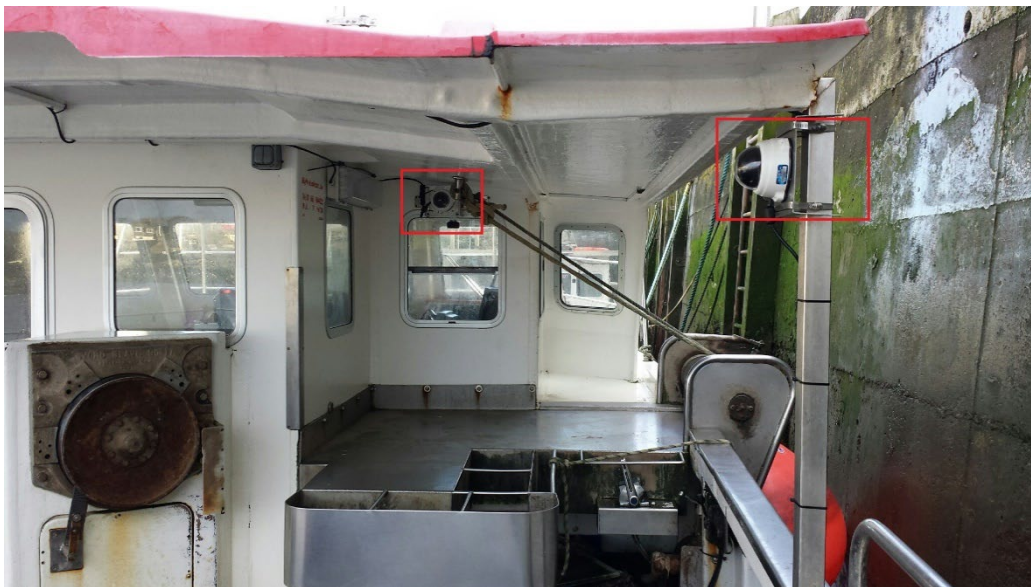
Figure A2 - CCTV cameras installed on an inshore creeling vessel.
